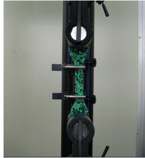
Fig. 5. Tensile strength test
