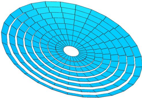
Fig. 2. Design of fresnel solar collector dish
