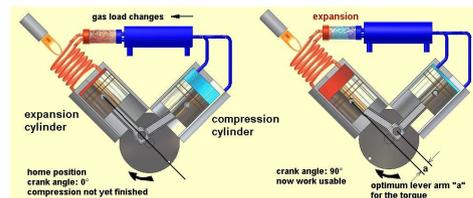
Fig. 1. Stirling Engine basic principle of motion[10]
