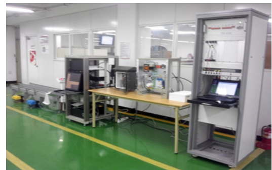
Fig. 18. Test Bed for Axle Counter test
