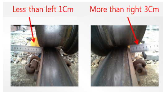
Fig. 13. Axle range out of rail
