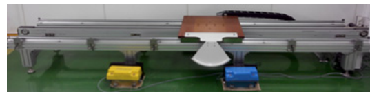
Fig. 17. Imitation axle moving system for test
