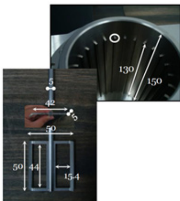
Fig. 6. Dimension of the BMC, in mm
