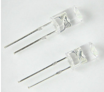
Fig. 2. LED of Water-Clear Type
