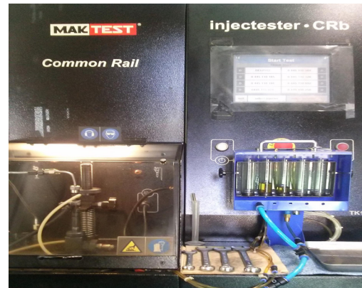
Fig. 8. Injector test machine
