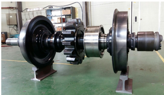
Fig. 12. Assembly of traction shaft
