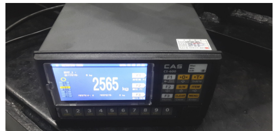
Fig. 17. Measuring system for band braking force
