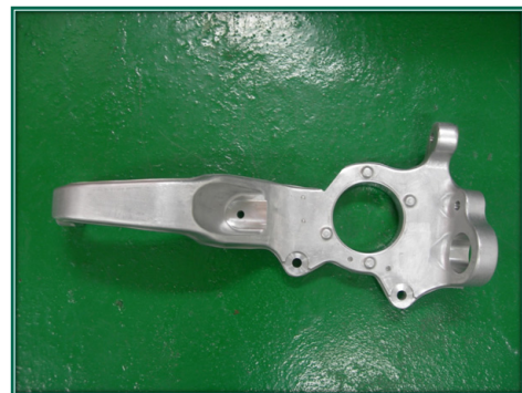
Fig. 8. Prototype of knuckle made by AA6061-T7 materials.
