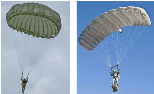
Fig. 1. Parachute (circular and ram-air type)
