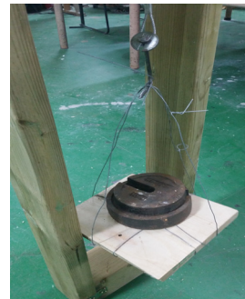
Fig. 6. View of Applied Load as Cable Tension
