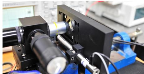
Fig. 11. Accuracy test of grid moving mechanism
