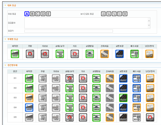
Fig. 9. Identify current status of bridge through mobile inspection Application
