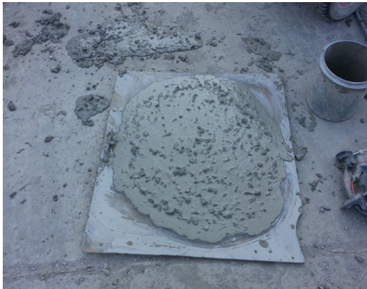
Fig. 4. Segregation of Concrete adding Copper Slag 40%
