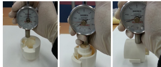
(b) 3D printed components (ABS, Shore D = 74.3)
