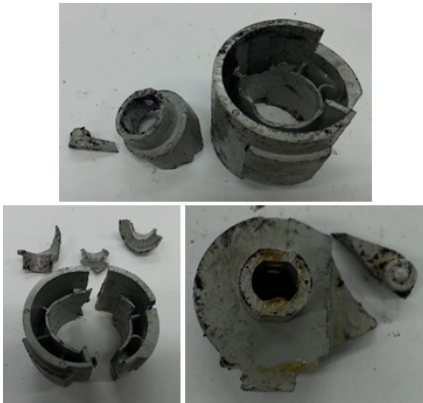
Fig. 4. Breakdown results of hub-driven and lever lockup components (PVC material, Injection molding process)
