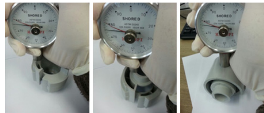
(a) Original component (PVC, Shore D = 78.6)
