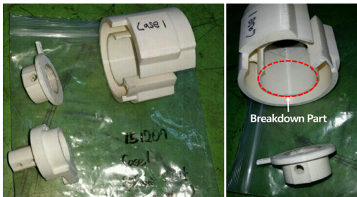
Fig. 10. Experimental results of 3D printed components (FDM method, ABS material)
