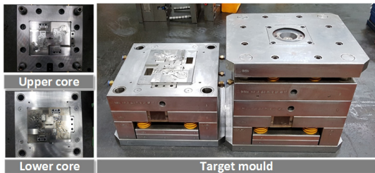
Fig. 16. Mould for injection moulding experiments
