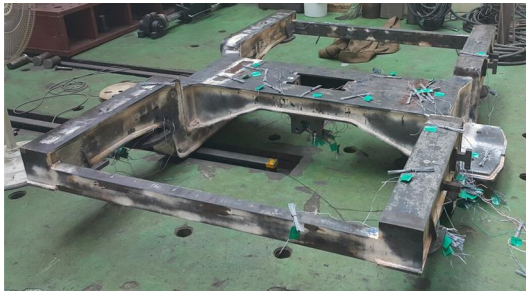
Fig. 6. Completed bogie frame
