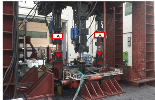
Fig. 8. Application of vertical loads to the bogie frame on the loading frame
