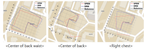
Fig. 12. Experimental results with regard to PDR module's mounting position
