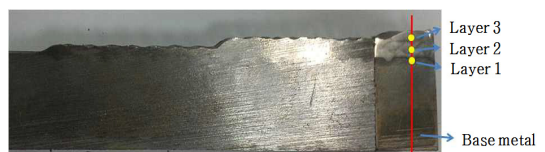
Fig. 10. Specimen of pipe overlay welding
