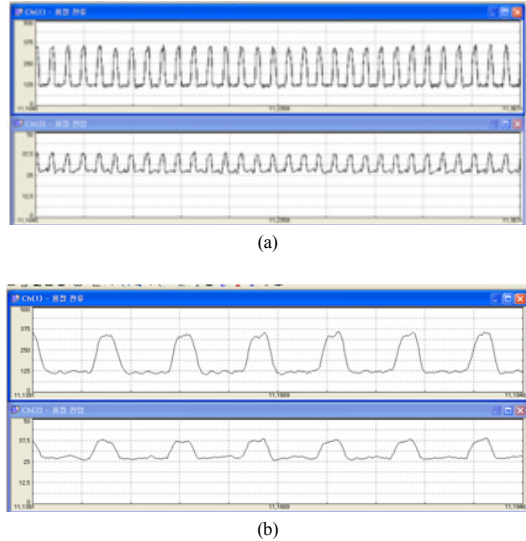
Fig. 4. Waveform of the current and voltage (a) Pulse waveform for comparison analysis (b) Distended pulse waveform
