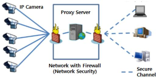
Fig. 2. Remote Access Method using Proxy Server
