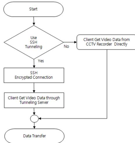
Fig. 4. Connection Algorithm
