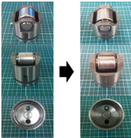
Fig. 14. Endurance test result of tappet housing
