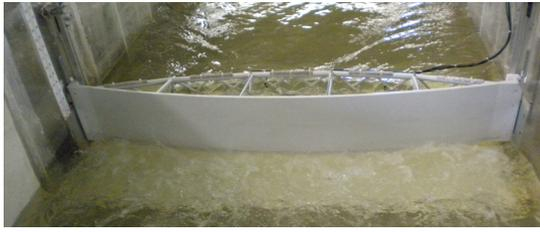
Fig. 3. Photo of gate model test
