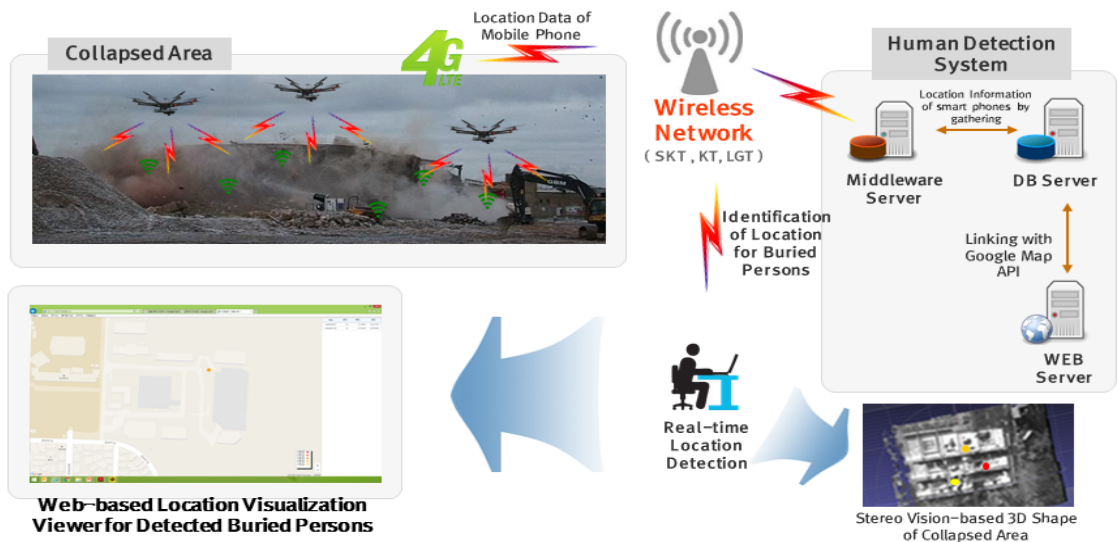
Fig. 2. An overall framework of burial location representation by a wireless communication-based human detection module with UAV
