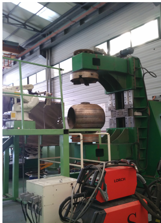
Fig. 1. Configuration of Overlay Welding Automation System for Ball-valve
