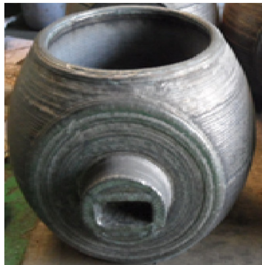
Fig. 15. Ball shape after overlay welding
