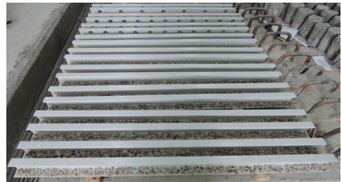
Fig. 3. Sand coated FRP planks
