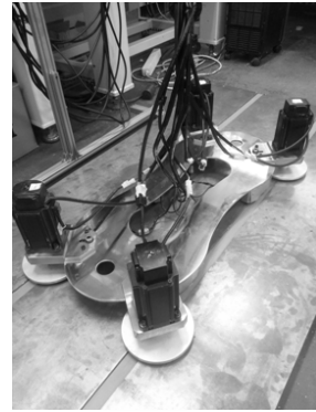
Fig. 10. Photograph of the conveyance system using electrodynamic wheels
