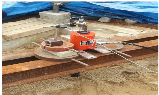
(c) Penetration Driver and Torque Measurement device
