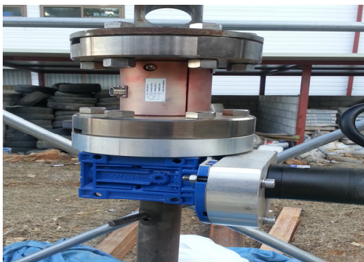
(b) Anchor and Instrumentation Jig for Anchor
