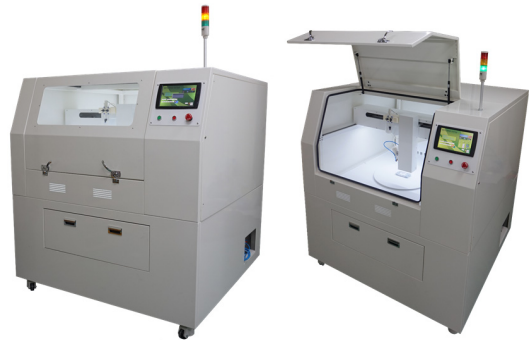
Fig. 2. 3D auto surface preparation system
