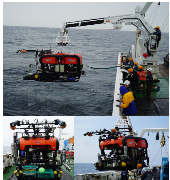
Fig. 1. Deployment and recovery of ROV ‘HEMIRE’.
