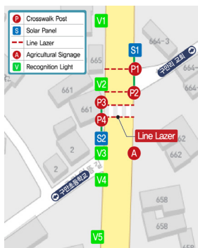
Fig. 13. Test-bed Installation Plan
