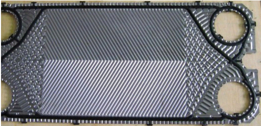
Fig. 1. Shape of titanium plate heat exchanger showing various pattern shape and gasket [1]
