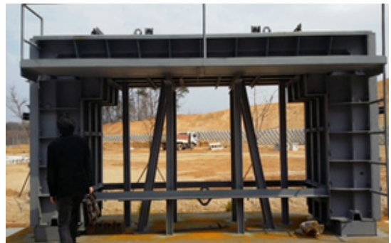
Fig. 1. PC BOX Form for Steam Curing
