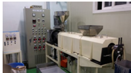
Fig. 2. Photo of small extruding machine
