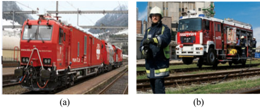
Fig. 2. Foreign fire fighting train (a) and unimog vehicles (b) for railway tunnel fire
