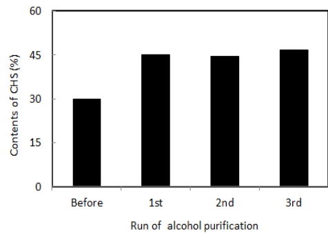
Fig. 4. Chondroitin sulfate content of skate cartilage with the number of ethyl alcohol purification. (CHS: Chondroitin sulfate)
