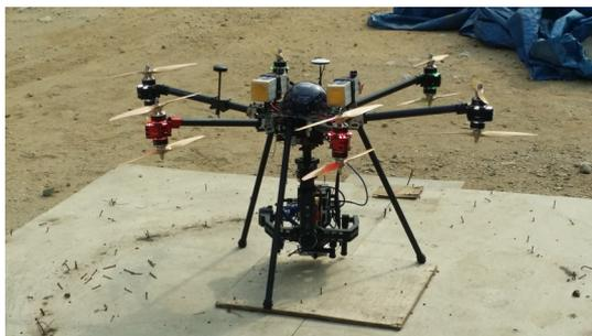
Fig. 4. Stereo Vision-based Drone
