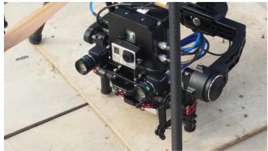
Fig. 5. Stereo Vision Camera Module
