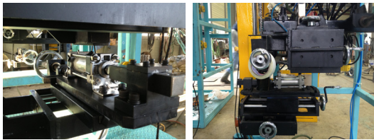
Fig. 13. Welding carriage equipment
