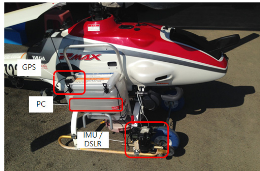
Fig. 1. Installing capturing equipment on UAV
