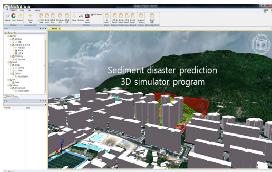
Fig. 14. Sediment disaster prediction 3D simulator programme
