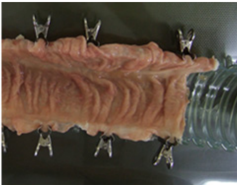
Fig. 4. in vitro test environment for locomotion of rotational inertial type robot
