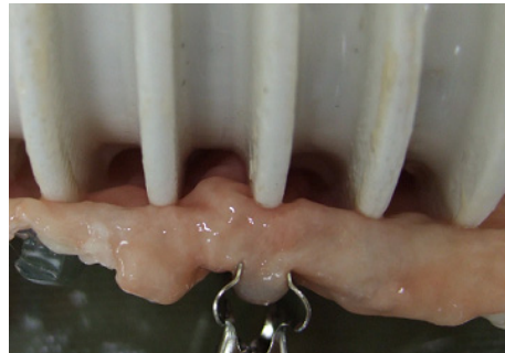
Fig. 5. winding up between colon wall and fin of robot occurs when screw angle becomes small
