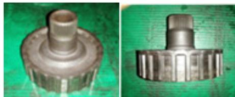
Fig. 3. Reaction hub of automatic transmission
