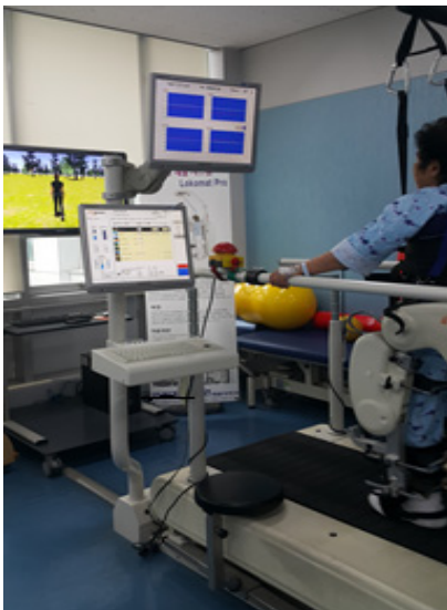
Fig. 1. Robot assisted gait training using Locomat ®
