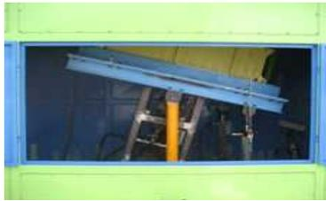
Fig. 2. Test Bed for Sloshing[10,11]
