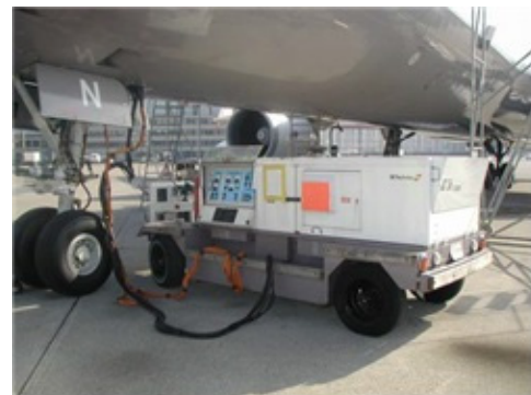
Fig. 10. GPU for electrical power [11]
