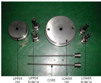
Fig. 11. Shaping process mold
