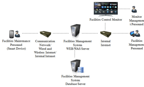
Fig. 11. Total System Diagram of Urban Facilities Management
