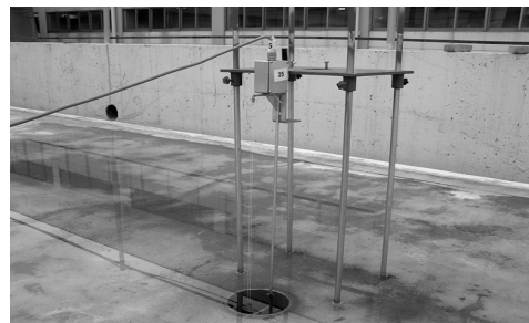
Fig. 5. Installation of wave height meter
