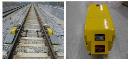
Fig. 1. Complete view of installed HBD sensor
