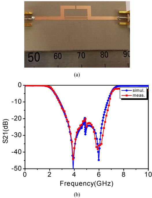
Fig. 5. A Photograph of the fabricated bandstop filter with dual spurline (a) Fabricated the bandstop filter (b) S-parameters( $S_{21}$ )
