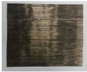
Fig. 9. Metal-coated carbon fiber electromagnetic wave shielding film
