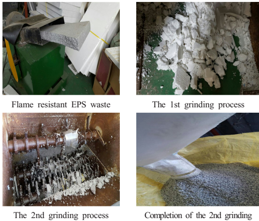
Fig. 2. Flame resistant EPS waste grinding process
